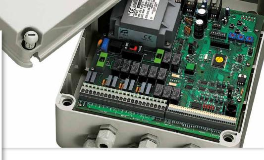
A wide range of telemetry receivers have been designed for outdoor Pan & Tilt remote control, which includes the most basic to the most complete models, and enable Pan & Tilt function management and motorised lenses.
