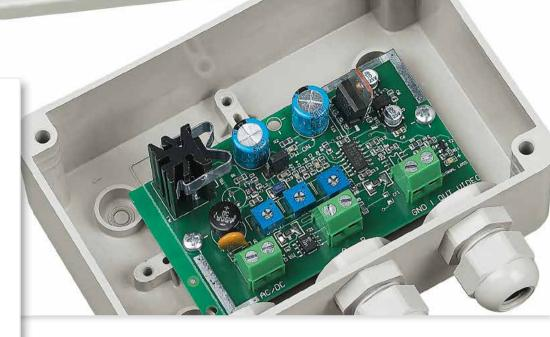
Videotec video transmission devices comprise pair cable transmitters/receivers to send longdistance signals.
